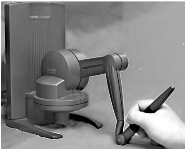
Figure 1 The Laparoscopic Impulse Engine is a simulated surgical grasper. The realistic tool handle is used to grasp simulated tissue. The tool can be rotated around a fulcrum and can be inserted or pulled back. Force is felt in 2 rotational and one translational direction.
