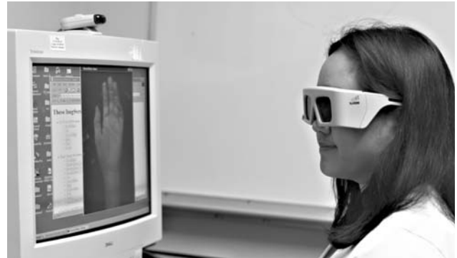
Figure 2 The polarized glasses have a wireless or wired connection to the infrared emitter box, which is usually placed on top of the computer screen.
