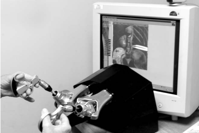
Figure 8 Bimanual surgical manipulators that control virtual tools in the simulation. Each manipulator can translate in and out of the trochar, and has pitch, yaw and twist movement, with haptic feedback on each of these axes. Pinch forces are felt when the grip is closed. An additional twist freedom is provided to allow the tool handle to rotate with respect to the rest of the tool.
